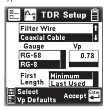
From the TDR Menu, press the Setup key to enter the TDR Setup.
